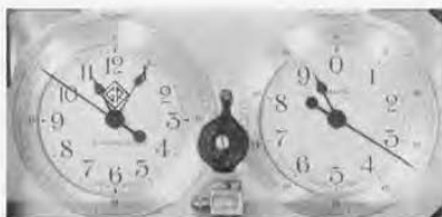
FIGURE 2. The dial of the high-speed stroboscopic clock. The right-hand dial carries two hands, the shorter rotating once each second, the longer ten times per second
